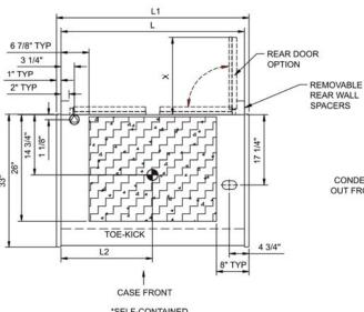
\*SELF-CONTAINED SERVICE ACCESS AREAS ONLY ACCESSIBLE BY PULLING OUT COMPRESSOR UNIT
