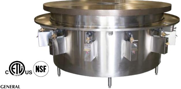
This specification lists the standard and optional features of Town Mongolian Barbecue ranges. Town MBR units feature multiple burners, each controlled by individual gas valves. This allows for maximum heat control of the cooking surface, low gas consumption during off hours and a fail safe if a burner should fail during operation. All burners have a pilot flame failure device that shuts off gas flow to a burner if a pilot light fails.
