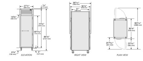
Electrical U.S. International Horsepower 3⁄4 N/A N/A Amps 8.7 115/60/1 Voltage NEMA 5-15P Cord Length 9 ft. 2.74 M. U 115/60/1 NEMA-5-15R
