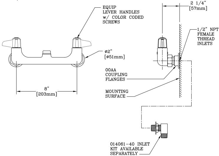
NOTE: ROUGH-IN REQUIREMENTS ø1" [ø25mm] HOLES 8" [203mm] ON CENTER
