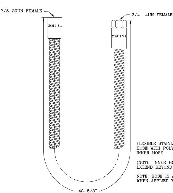
FLEXIBLE STAINLESS STEEL HOSE WITH POLYURETHANE
