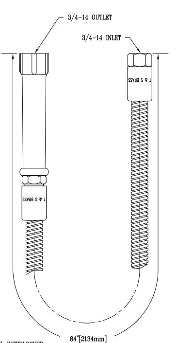
FLEXIBLE STAINLESS STEEL INTERLOCKED OUTER COVER WITH REINFORCED POLYURETHANE INNER HOSE
