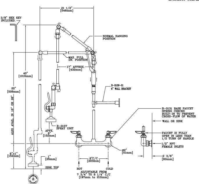
NOTE: ALSO AVAILABLE WITH 1/2" NPT MALE INLETS AND LOCKNUTS ON FAUCETS IN PLACE OF FEMALE INLETS.
