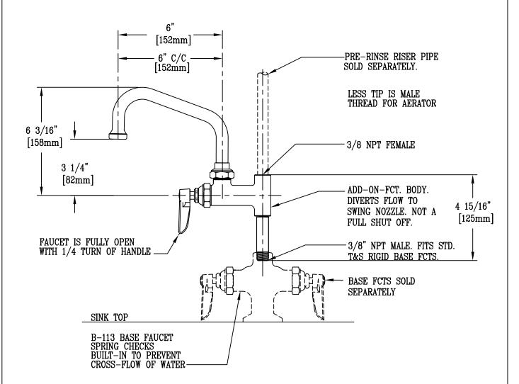
NOTES: THE ADD-ON FAUCET IS AN ADDITION TO PRE-RINSE UNITS AND IS INSTALLED IN OUTLETS OF BASE MIXING FAUCETS OF UNITS BEFORE FITTING RISER PIPE, AS SHOWN.
