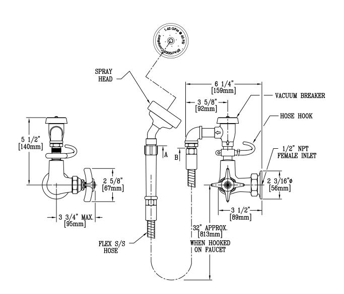
STANDARD HOSE LENGTH FROM A TO B IS 68", BUT CAN BE MODIFIED TO ANY LENGTH.
