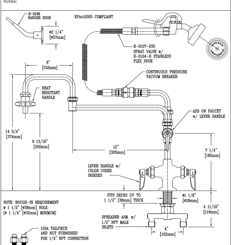
Product Description: DECK MOUNT MIXING FAUCET w/ B-0107-035 SPRAY VALVE, 18" DOUBLE JOINT SWING NOZZLE, 104" FLEX HOSE & ADD ON FAUCET
