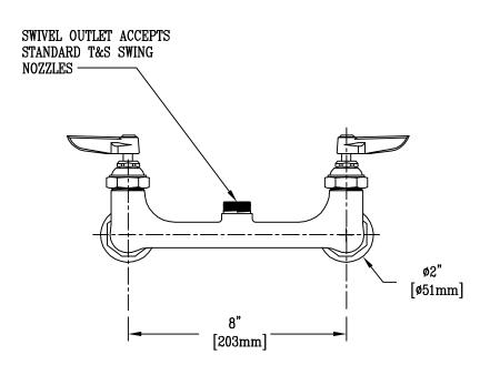
8" c/c WALL MOUNT MIXING FAUCET LESS NOZZLE, AND WITH 1/2" MALE "EE" INLETS
