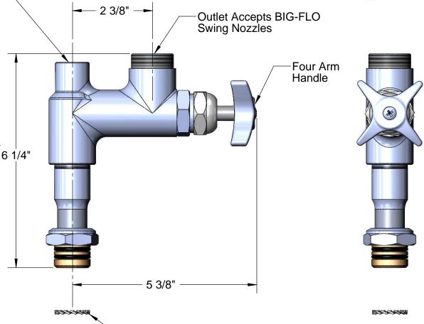
Furnished with Serrated Lock Washer for Non-Swivel Installation in Base Faucet
