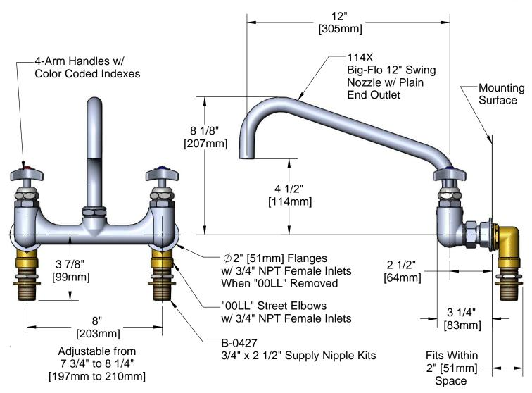
Rough-In:  $\emptyset$ 1 1/4" [32mm] Holes in Mounting Surface.
