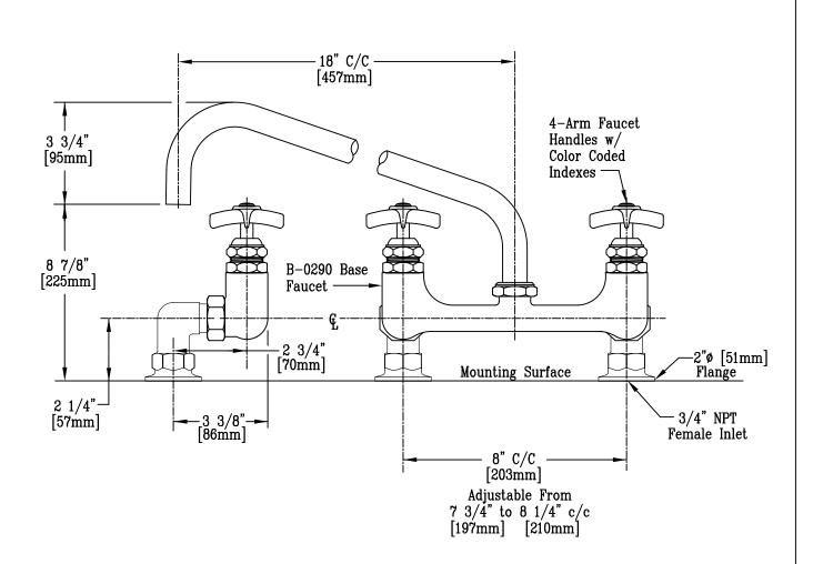
Note: Drill 1 1/4 % [32mm] Holes on 8 % c/c in Mounting Surface.
