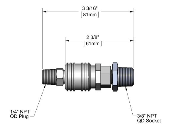
When 1/4" NPT Plug is removed from QD Socket, flow is automatically shut off.
