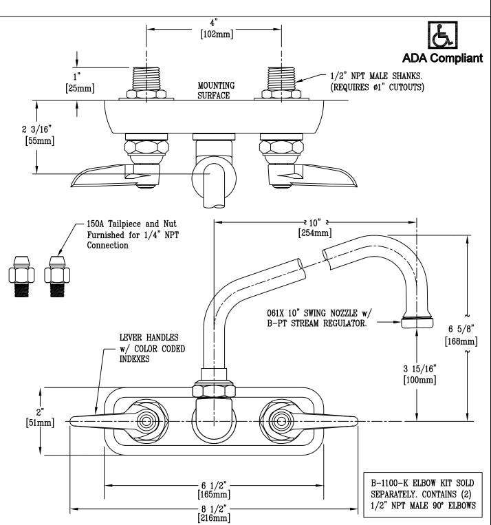
Product Description: WALL MOUNT WORKBOARD FAUCET WITH 1/2" NPT MALE SHANKS, 4" INLET CENTERS, 061X 10" SWING NOZZLE, B-PT STREAM REGULATOR & LEVER HANDLES
