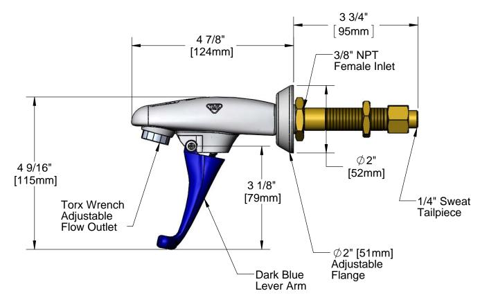
Note: Nipple Shown Allows B-1202 Glass Filler to be Fitted to a 2-1/4" [57mm] Max. Thick Cabinet. Also
