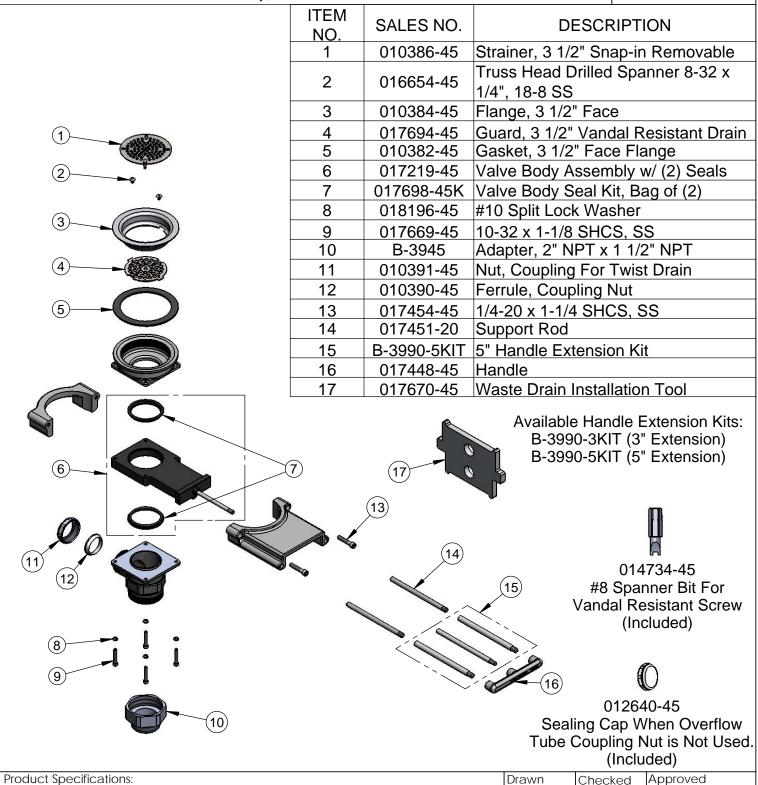
Modular Waste Drain Valve w/ Pull Handle, 3 1/2" Sink Opening, 2" NPT Female x 1-1/2" NPT Male Adapter, 5" Handle Extension
