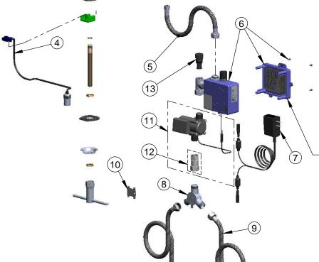
A maximum of (8) ChekPoint Faucets can be hardwire connected and powered by ChekPoint Hardwire AC Transformer. EC-HARDWIRE (Sold Separately)
