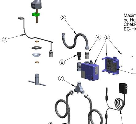
Maximum of (8) ChekPoint Faucets Can be Hardwire Connected and Powered by ChekPoint Hardwire AC Transformer. EC-HARDWIRE (Sold Separately)
