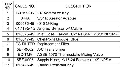
Maximim of (8) ChekPoint Faucets Can be Hardwire Connected and Powered by ChekPoint Hardwire AC Transformer EC-HARDWIRE (Sold Separately)
