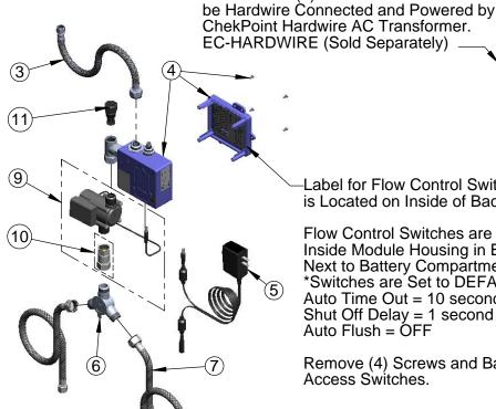
Label for Flow Control Switch Settings is Located on Inside of Back Cover.
