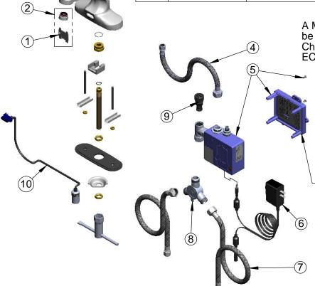
A Maximum of (8) ChekPoint Faucets Can be Hardwire Connected and Powered by ChekPoint Hardwire AC Transformer. EC-HARDWIRE (Sold Separately)
