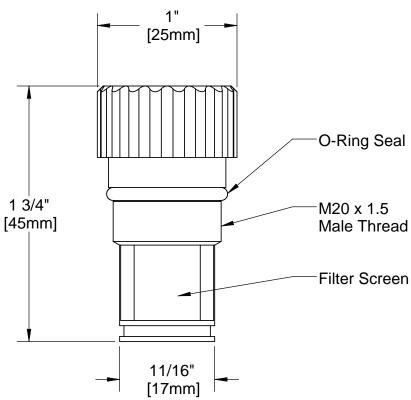
Approved Drawn Checked **Product Specifications: GEF JRM JHB** ChekPoint Replacement Control Module Filter Date: Scale: 3:2 3/30/09
