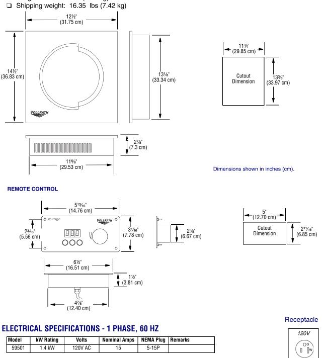
□ Electrical Connection: Requires a 15A circuit. Unit supplied with a NEMA 5-15P plug.
