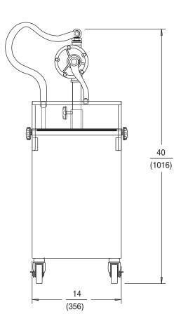
NOTE: Specifications are subject to change without notice. This system is designed to pump and discard old oil only and only when below 100°F (38°C). Never attempt to pump any hot liquid (above 100°F) with this oil caddy. Failure to follow this warning may result in serious burn injury. Always tighten pump pipe knob before pumping oil. NEVER USE THIS SYSTEM TO PUMP WATER OR CHEMICALS.
